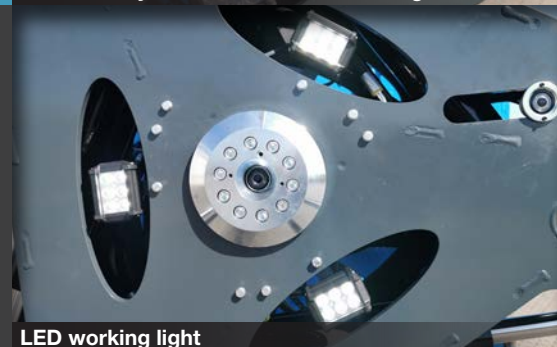
2 Camera System - for hub and bolt alignment
