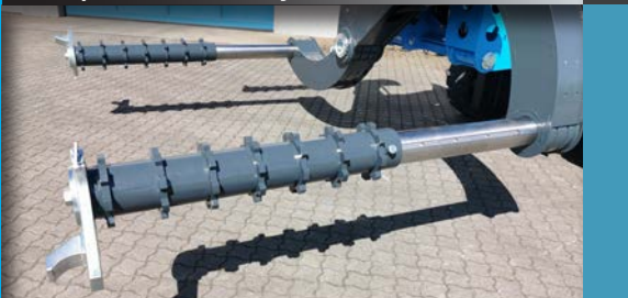
Telescopic pipes for long reach
