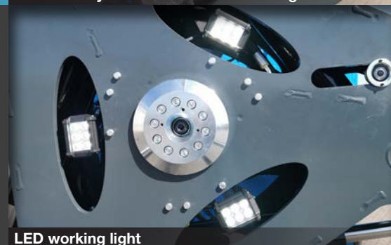
2 Camera System - for hub and bolt alignment
