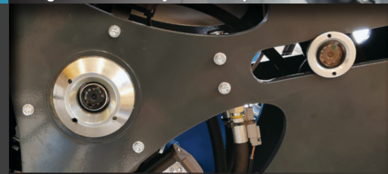
Optional second camera for precise bolt alignment
